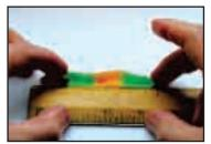
Stretch the snake by a set amount of time, release and leave for a minute to contract, and then re-measure. Repeat increasing the stretch amount by 10% of the original length each time until the snake breaks.
