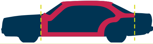
Figure 2 Passengers sit inside the rigid passenger cell, shown in red. Crumple zones are the parts in front of and behind the cell. They are designed to be weak, so that they crumple and absorb the energy of an impact. Games designers must make their on-screen cars collapse in a convincing way
