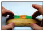
Stretch the snake by a set amount of time, release and leave for a minute to contract, and then re-measure. Repeat increasing the stretch amount by 10% of the original length each time until the snake breaks.
