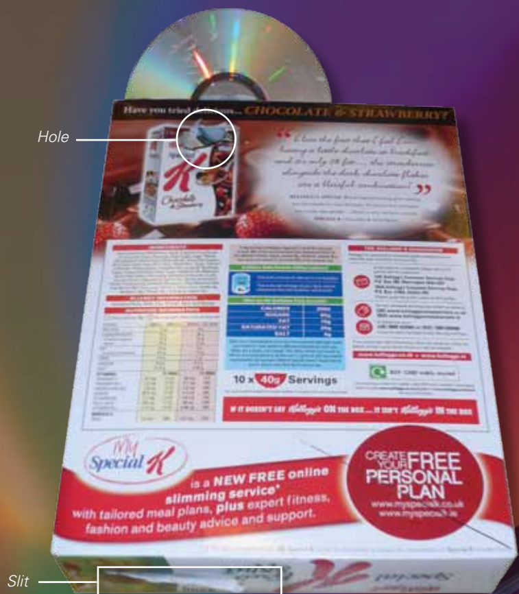
The cereal box spectroscope
